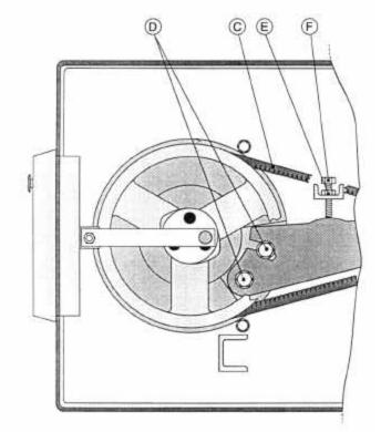
1. Start by tightening the V-belts (C).
